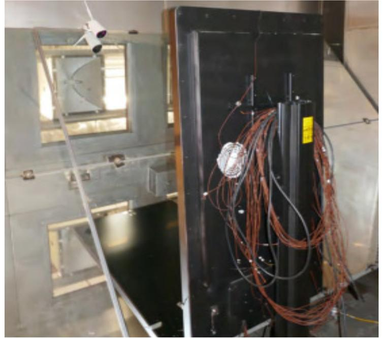
In order to properly test the monitors, they needed to be mounted upright, just as they would be when used in a normal application. Because the lights in the solar chamber are directly overhead, the testing engineers had to get creative. The team utilized mirrors to redirect the light radiation towards the front screen while maintaining the proper orientation for gravitational effects.
