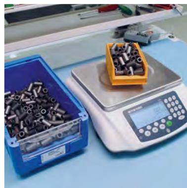
Measure accurate quantities for shipment and create labels for production with counting scales.
