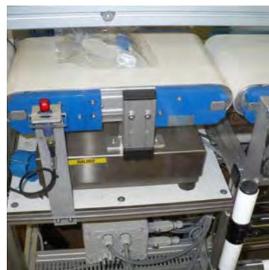
In-line checks with weighing platform.
