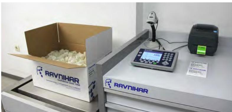
Counting station on shop floor, barcode scanner to start an operation and to load article data and package counts and a printer to supply labels for identification and transportation.
