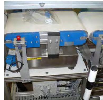
In-line checks with weighing platform.
