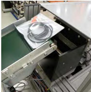
Belt feeds package onto scale.
