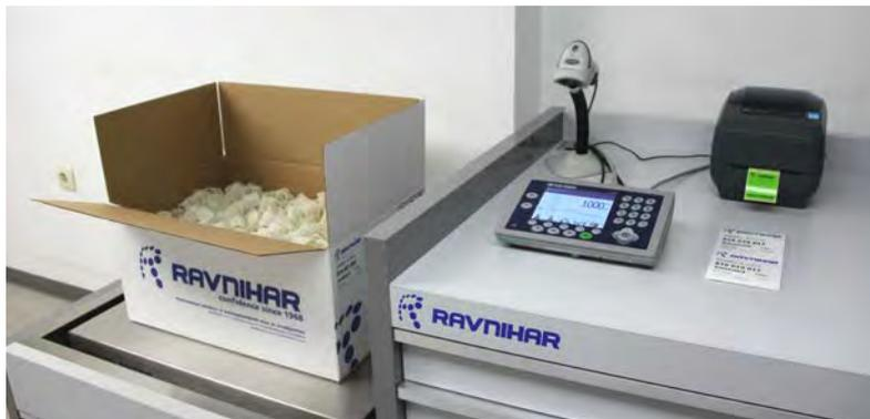
Counting station on shop floor, barcode scanner to start an operation and to load article data and package counts and a printer to supply labels for identification and transportation.
