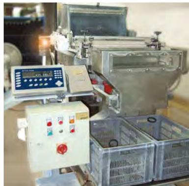
Scale terminal controls alarm light and material flow.
