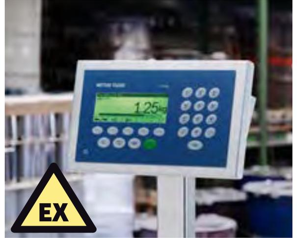
Installing intrinsically safe weighing equipment is the safest method to protect from explosion hazards. Intrinsically safe systems enable equipment to be used without risk of igniting any flammable gas, dust or fibers that may present in hazardous areas. Compared to other protection methods, such as flame-proof enclosures, intrinsically safe equipment is easy to handle and can be serviced without halting production.
