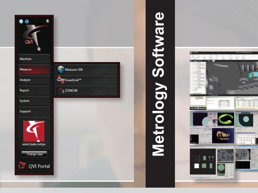
Portal Navigation Panel allows you to start or switch between QVI measurement applications, with no searching for icons on the Windows desktop.
