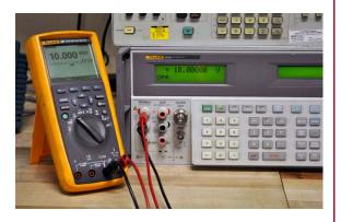
It is necessary to calibrate multimeters by checking multiple test points for each parameter, versus simply checking one test point per parameter. This ensures the multimeter is suitable for use throughout its full range of capabilities. <u>Click here</u> to learn more about the importance of multiple test points and J.A. King's multimeter calibration procedures.
