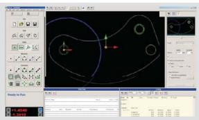
eChek provides full measurement and construction functionality for points, midpoints, angles, lines, arcs, circles, distances, widths, included angles, angle intersections, line/circle intersections, point-to-point distances, gage ball tangent to two lines, and gage ball between two non-parallel lines. Can be used manually or with automatic edge detection.
