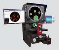
Patented eCAD® projects an accurately magnified CAD model directly onto the comparator screen, presenting a virtual chart gage, including nominal dimensions and tolerance bands.
