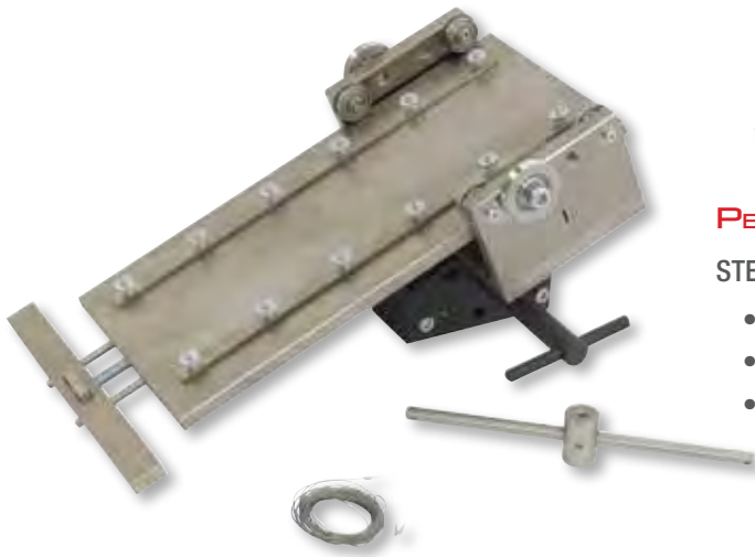
Shown: PEEL-50MS-1 model with adjustable angle platform.
