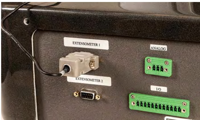
Analog and Digital I/O Termination Panel Shown on MMS and MMD Material Test Frames (MMD-50K)
