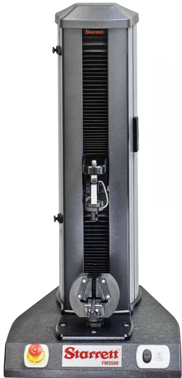
MMS-500 Series shown with optional load cell sensor and bottom test fixture
