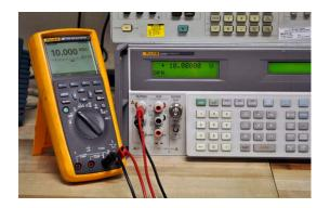
It is necessary to calibrate multimeters by checking multiple test points for each parameter, versus simply checking one test point per parameter. This ensures the multimeter is suitable for use throughout its full range of capabilities. Click here to learn more about the importance of multiple test points and J.A. King's multimeter calibration procedures.
