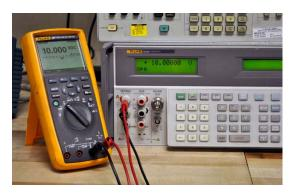
It is necessary to calibrate multimeters by checking multiple test points for each parameter, versus simply checking one test point per parameter. This ensures the multimeter is suitable for use throughout its full range of capabilities. Click here to learn more about the importance of multiple test points and J.A. King's multimeter calibration procedures.
