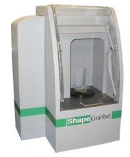
Checking such complex parts using a few sample points collected with a caliper or even a CMM is time consuming and doesn't provide a complete inspection. ShapeGrabber 3D laser scanners speed up the inspection process while providing additional data.
