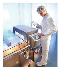
In addition to new equipment sales, J.A. King also now offers metal detector calibration at all of our full service locations. All HACCP-based standards require regular monitoring of metal detector effectiveness. For complete peace of mind, a third party calibration backs up your daily checks and ensures your equipment is functioning properly.
