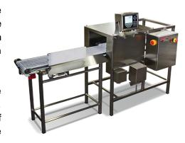
And don't forget to have your checkweigher regularly calibrated so you can provide proof of its accuracy.
