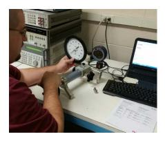
We can calibrate pressure devices up to 30,000 psi and low or differential pressure down to 28 inH<sub>2</sub>O. Calibrations can be performed in one of our 15 ISO 17025 accredited laboratories or on-site at your facility or job-site. We also offer in-process pressure calibrations services, and our technicians are accustomed to working in a variety of environments.
