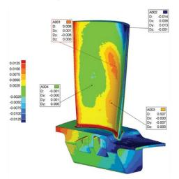
With ShapeGrabber 3D scanners, aerospace manufacturers can reduce inspection time (both first article and production) and greatly enhance part coverage.
