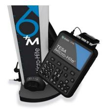
The MICRO-HITE and MICRO-HITE+M gages are available in both manual and motorized models with three different height options (350mm/ 600mm/ 900mm) to fit your specific needs. Other features include:
