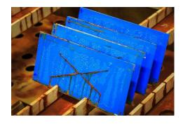
Take a look at our article about <u>Salt Spray Testing</u> for more in depth information including when not to use salt spray testing and the difference between Neutral Salt Spray (NSS) and Copper Accelerated Acetic Acid Salt Spray (CASS).
