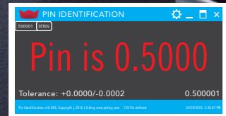
Fig 2. Failed Result: This is a ZZ-minus pin measuring 0.500001. Since the upper tolerance is 0 inches, the closest corresponding pin has a diameter less than what was measured and is noted in red.
