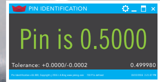
Fig 1. Positive Result: This is a ZZ-minus pin measuring 0.499980 inches. That is within the displayed tolerance (+0.0000/-0.0002) so the corresponding pin (0.5000 inches) is green, indicating that it passes.
