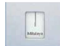
To measure resilient workpieces, take the measurement when the pointer is between the two index lines.
