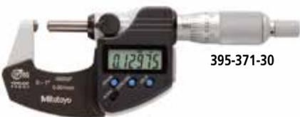
Digital model with spherical anvil
