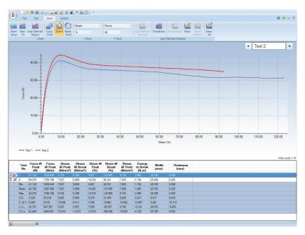
ASTM D 204 Test methods for sewing thread.
