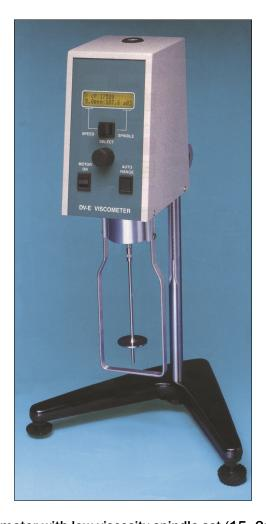
**KFG-2291:** Digital Viscometer with low viscosity spindle set (15–2m)
