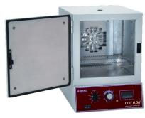
Ideal for colorfastness to perspiration and water tests. Digital temperature display with 0.1dgs C resolution, maximum temperature 90 dgs C, excellent temperature stability and uniformity. Metal door with magnetic latch, 2 stainless steel shelves included.
